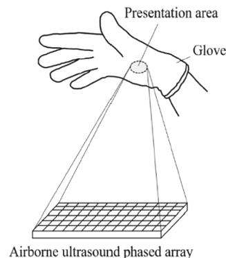
**Fig. 6 A hand wearing a cloth glove can be heated remotely by focusing ultrasound waves [15].**
