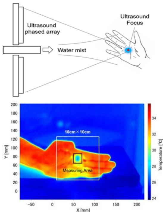
**Fig. 5 Display of a pin-point cooling sensation by ultrasound focus in water mist [13].**
