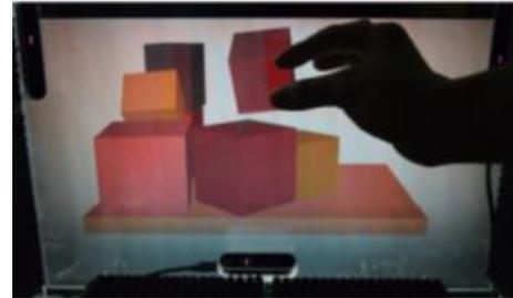
Fig. 1 Ultrasound haptic feedback is provided depending on the status of contact with virtual objects. [3].
