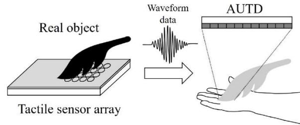
**Fig. 3 A microphone array records the vibration when an object is traced over it, which is then reproduced by a transducer array [9].**
