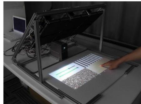
**Fig. 4 Focusing the ultrasound waves at the point where the finger touches reduces the frictional force [12].**
