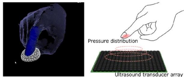
Fig. 2 The pressure distribution on a finger touching a soft object is reproduced by a transducer array [6].
