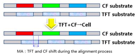
Fig. 15. The schematic diagram of MA
