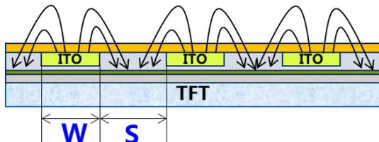
Fig. 4 The schematic diagram of ITO\_W/S
