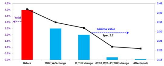
Fig. 19. Yield rate improvement in practical applications, the abscissa is the introduction of different countermeasures (Before: Countermeasures not introduced; After(input): Introduction of countermeasures for ITO\_W/S+PI\_THK changes)
