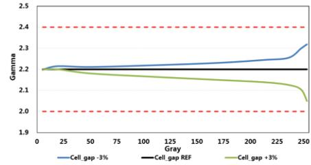
Fig. 12 The influence of Cell gap by simulation
