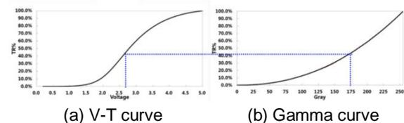
Fig. 1 The relationship between grayscale and voltage of LCD
