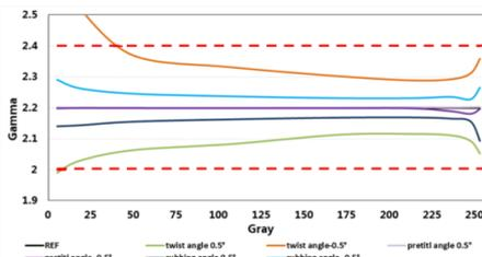
Fig. 17. The influence of Twist angle, Pretilt angle and Rubbing angle by simulation
