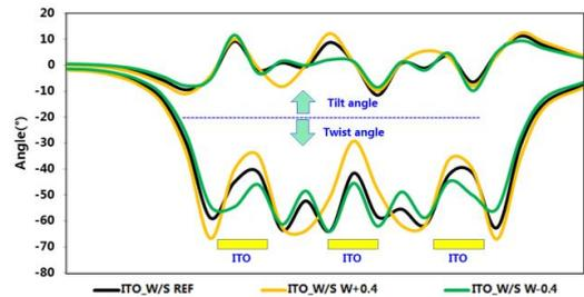
Fig. 6 Simulation of Tilt angle and Twist angle for different ITO\_W/S
