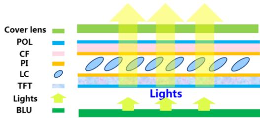
Fig. 2. Display model for Gamma simulation
