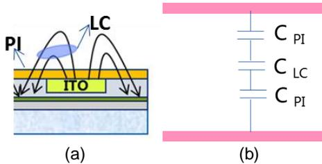
Fig. 9 Equivalent circuit of LC and PI
