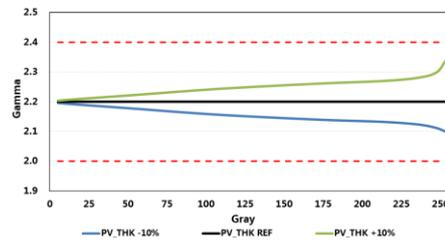
Fig. 14 The influence of PV\_THK by simulation
