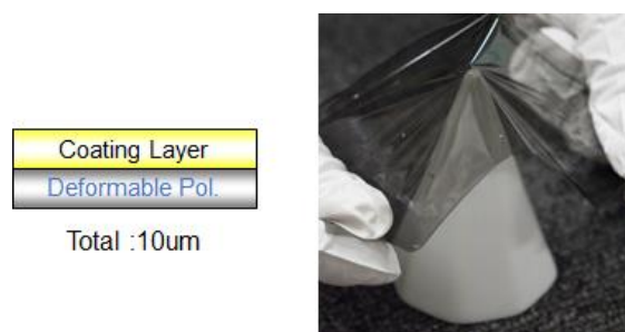
Fig. 2 Configuration & photograph of the deformable polarizer
