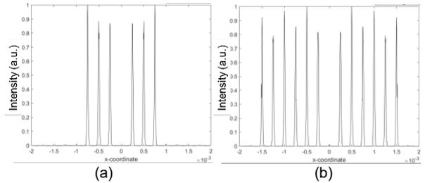
Fig. 3. The simulation resulted profiles of (a) 1x6 and (b) 1x12 switches only using the IFTA algorithm.
