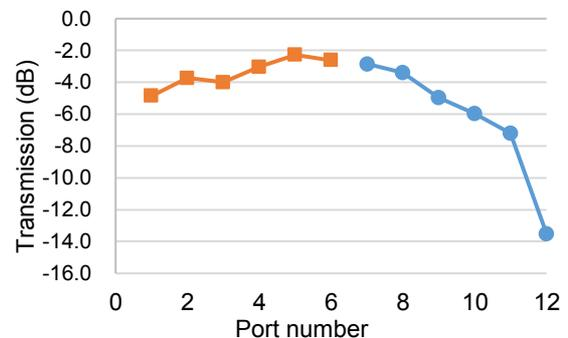
**Fig. 6. Transmission of 1 x 12 optical switch deflection to single port in this study.**
