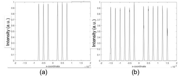
Fig. 4. The simulation resulted profiles of (a) 1x6 and (b) 1x12 optical switch using the optimization method proposed in this study.
