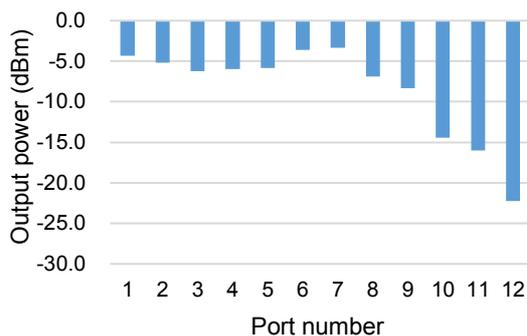
**Fig. 7. The energy corresponding to different output ports of the optical switch multicast to 12 ports in this study.**
