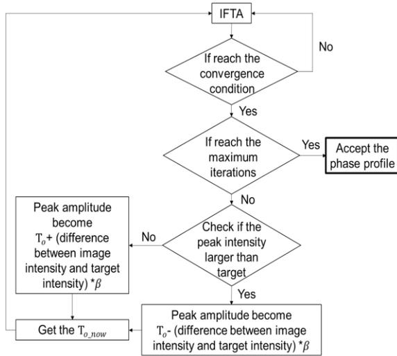
Fig. 2. Flow chart of uniformity optimization algorithm.
