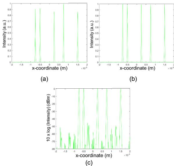
**Fig. 5. The simulation resulted profiles of deflecting to any five fibers (a) only using the IFTA algorithm, (b) and (c) using the optimization method proposed in this study.**
