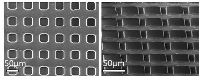
**Fig. 5 SEM images of coalesced GaN platelets, from above (left) and with a tilted view (right)**
