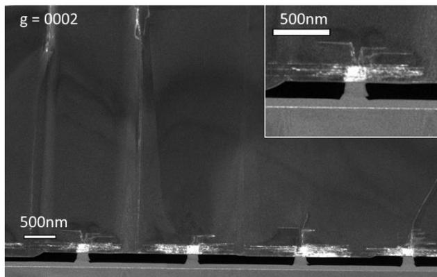
**Fig. 4 TEM cross-section image of coalesced nano-pyramids, with zoom of broken nano-pillar (inset)**
