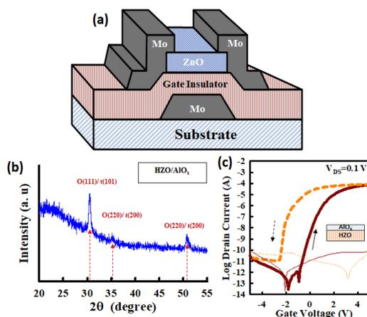
**Fig. 1** (a) Schematic cross-sectional view of the fabricated ZnO TFT with a ferroelectric gate insulator. (b) GI-XRD spectra of HZO/AlO<sub>x</sub> films on glass. (c) Transfer characteristics with hysteresis and corresponding leakage current of spray coated ZnO TFTs on stack HZO/AlO<sub>x</sub> gate insulator.
