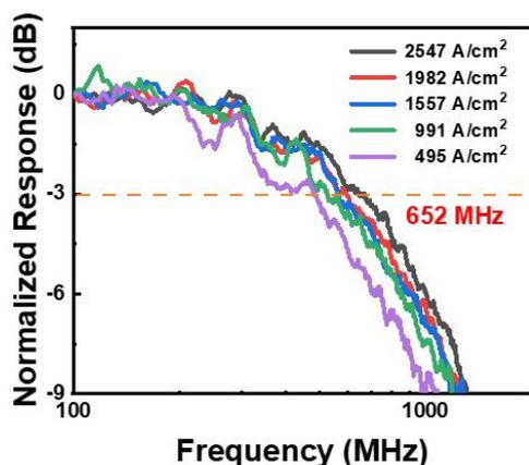
**Fig. 2** Frequency response for semipolar blue  $\mu$ -LED.
