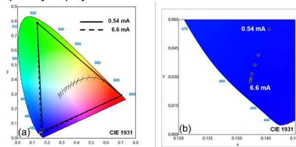
**Fig. 3** Color performance of semipolar  $\mu$ -LED under various injection current on the CIE 1931 color space diagram. (a) The color gamut of full-color display device. (b) Color coordinates of semipolar  $\mu$ -LED.
