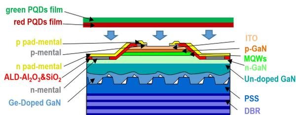
**Fig. 1** Schematic diagram of full-color display device
