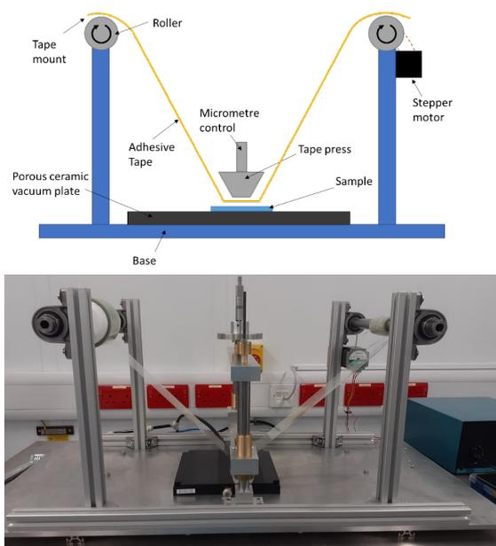
**Fig.2 Schematic diagram (top) and photograph (bottom) of the adhesion lithography tool.**
