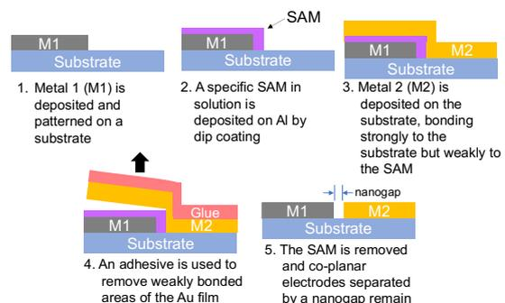
**Fig.1 Schematic diagram of the adhesion lithography process.**
