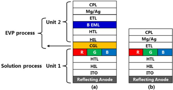
**Fig. 1 Architecture of (a) top emission RGB hybrid tandem OLED and (b) single unit RGB OLED.**
