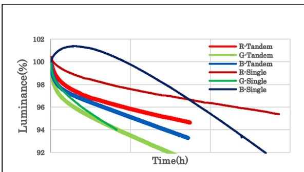
**Fig. 4 Lifetime of hybrid tandem device and single unit device.**
