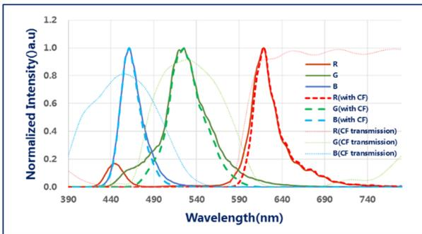
**Fig. 3 Graph of spectra of R/ G/ B hybrid tandem device treated with and without R/ G/ B CF transmission spectra respectively, and R/ G/ B CF transmission spectra.**
