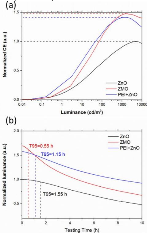
**Figure 4. The comparison of blue QLED performance between different ETL layer modification device. (a) relative current efficiency of different ETL layer modification device; (b) relative operational lifetime of different ETL layer modification device;**
