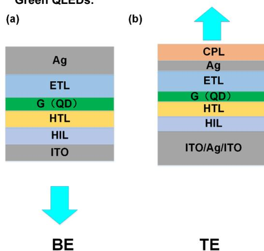
**Figure 1. Device structures of green QLEDs. (a) bottom emitting device structures, (b) top emitting device structures.**
