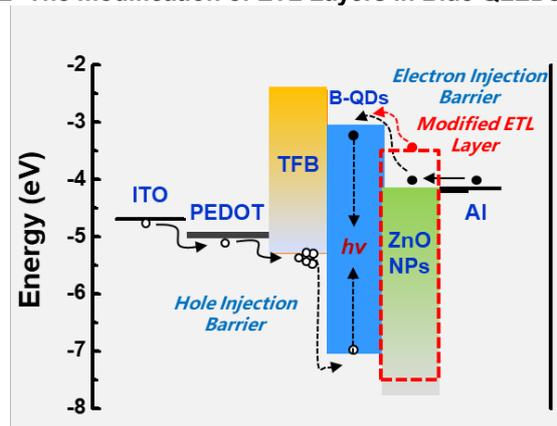
**Figure 3. Schematic energy level diagrams of the standard blue QLED device with ZnO nanoparticles as electron transporting layer and the electron injection improved blue QLED device with modified ETL layer.**
