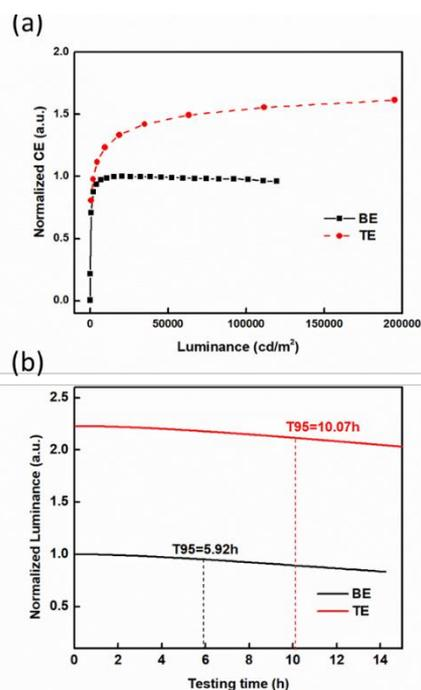
**Figure 2. The comparison of green QLED performance between TE and BE device structure. (a) relative current efficiency of TE and BE green QLED; (b) relative operational lifetime of TE and BE green QLED;**
