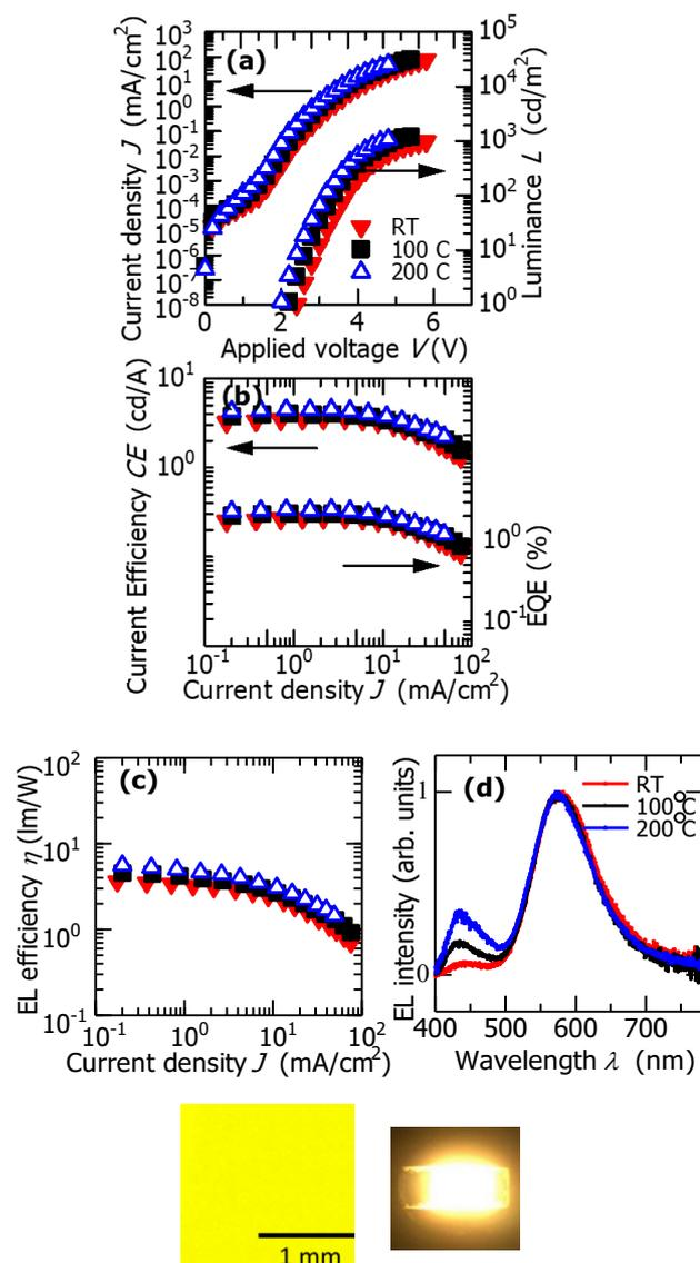
Figure 1: Characteristics curve of (a)  $J$ - $V$ ,  $L$ - $V$  (b)  $CE$ - $J$ ,  $EQE$ - $J$  (c) EL spectrum of fabricated QLED at different  $T_d$ .
