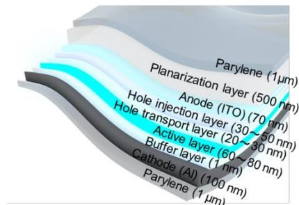
Figure 1. Structure of the ultra-flexible OLED
