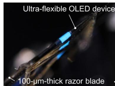
Figure 2. Picture of the ultra-flexible OLED
