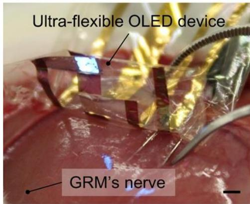
**Figure 3.** The OLED stimulator was attached to a surface of gracilis muscle (GRM) with high conformity, even during hindlimb movement.
