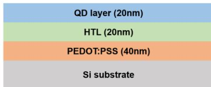
**Figure 1.** The sample structure for evaluation of morphology
