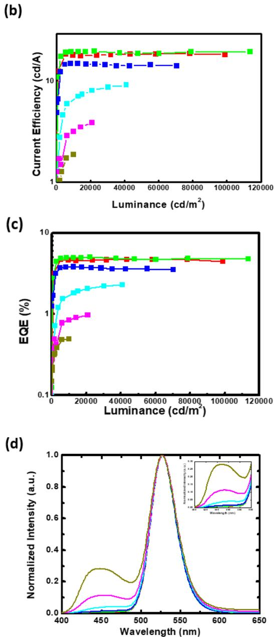
**Figure 4.** (a) Current density – voltage - luminance (*J-V-L*) characteristics, (b) Current efficiency – luminance, (c) external quantum efficiency (EQE) - luminance and (d) EL spectra of green emitting QD-only device and TCTA doped QD devices.
