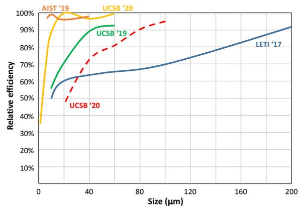
**Fig. 2 Drop in efficiency for small-size uLEDs. Solid lines: GaN-based blue LEDs, showing significant improvements at small size over time. Dashed line: GaAs-based red LED, which still suffer from significant size effects, even with good passivation. After data from [10-13]**
