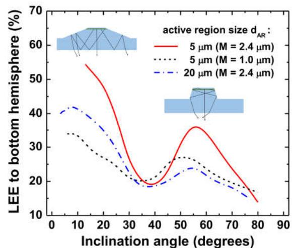
Figure 3 Modeled effect of a uLED’s shape on the light extraction efficiency, in a geometric-optics framework, showing the existence of ‘preferred angles’. Reprinted from [22] under CC license.
