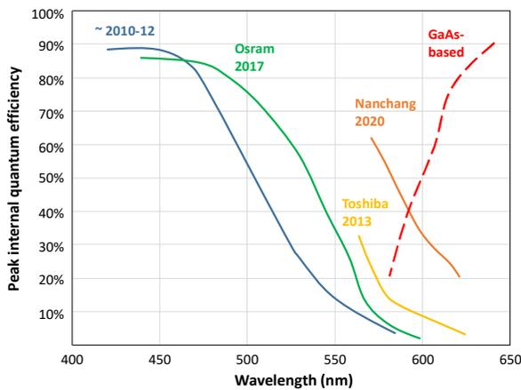
**Fig. 1 Evolution of the green gap. Full lines: efficiency of GaN-based LEDs over time. Dashed lines: GaAs-based long-wavelength LEDs. A decade ago, the green gap was pronounced; it is now slowly closing. After data from [15-18]**
