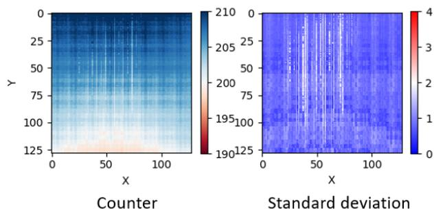
**Fig. 2 Delay offset distribution at each pixel**
