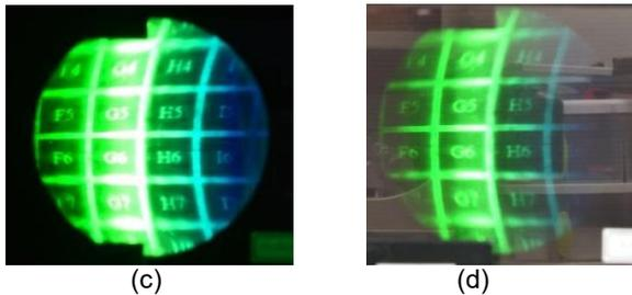
Fig4. The resulting image was performed with the green LED as the backlight. (a) the original pattern (3mm\*3mm per grid); (b) from the projected image at infinity; (c) Final image in the dark room; (d) Final image in the bright room.
