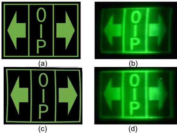
Fig5. The result of digital distortion correction was performed with an LC panel as the image source. (a) input image without correction; (b) final image without correction; (c) input image correction; (d) final image with correction.
