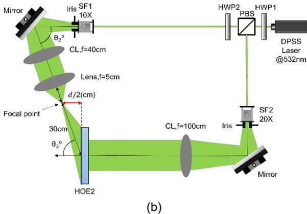
Fig 1. The optical system configurations were employed to record (a) HOE1 and (b) HOE2.
