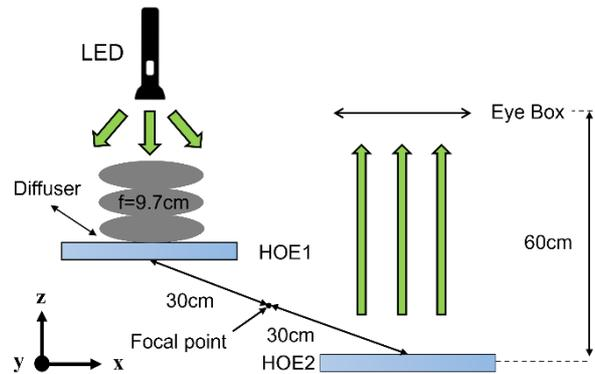
Fig 3. The dimension of the eye box was determined by measuring the image size of the aperture stop.
