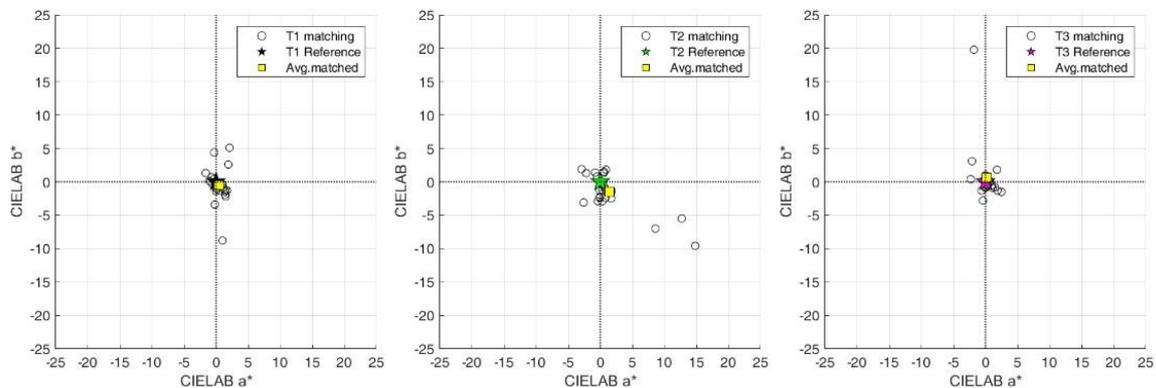
**Fig. 5 Color matching accuracy test results**
