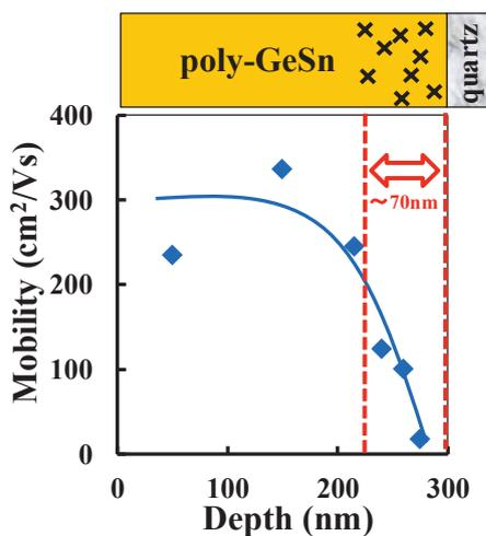
**Fig. 4 In-depth profile of carrier mobility for sample structure (i) with Sn concentration of 2%.[2]**
