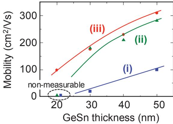
**Fig. 3 Thickness dependence of carrier mobility for sample structures (i), (ii), and (iii). Sn concentration is 2%.**
