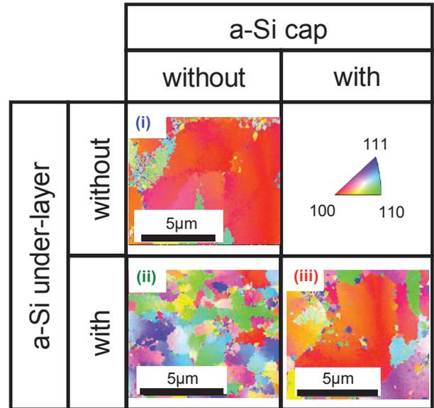
**Fig. 5 EBSD images of sample structures (i), (ii), and (iii) with GeSn thickness of 50 nm and Sn concentration of 2%.**
