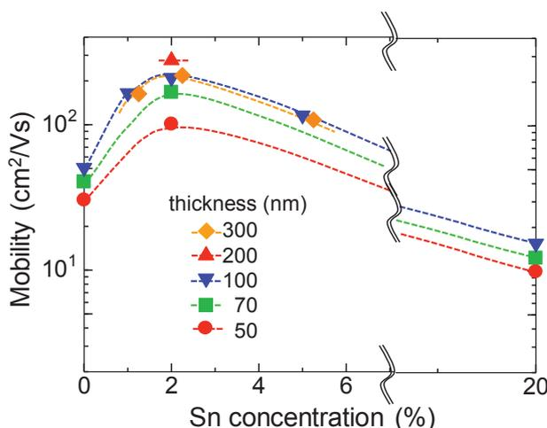
Fig. 2 Sn concentration dependence of mobility for sample structure (i).[2]
