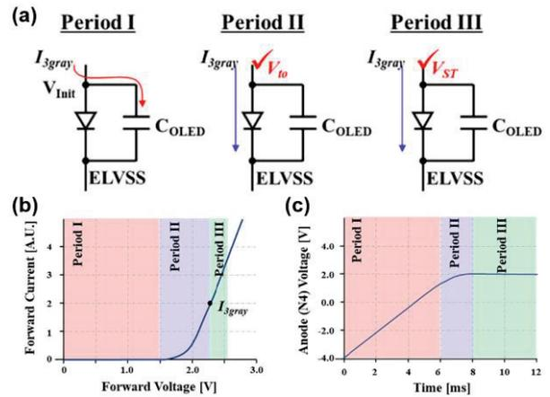
**Fig. 2. Schematics of OLED operation sequences based on a specific period. (a) Change of the conduction in equivalent circuit by 3 period, (b) OLED I-V curve by the operating period, and (c) anode voltage transition sequence [2].**
