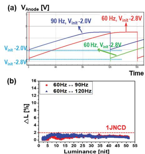
Fig. 5. (a) Simulation results for OLED anode voltage in various  $V_{init}$  at 60 and 90 Hz Conditions. (b) The differences in luminance under variable frequency changes with  $V_{init}$  compensation [3].
