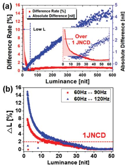
Fig. 4. (a) Differences in luminance between frequencies of 60 Hz and 120 Hz. (b) At low gray levels, differences in luminance under a frequency change from 60 to 90 Hz and 60 Hz to 120 Hz (without  $V_{init}$  compensation) [3].
