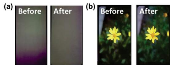
**Fig. 3. Improved result by minimizing of electric potential difference of anode: (a) low gray color uniformity and (b) low gray color crush [2].**
