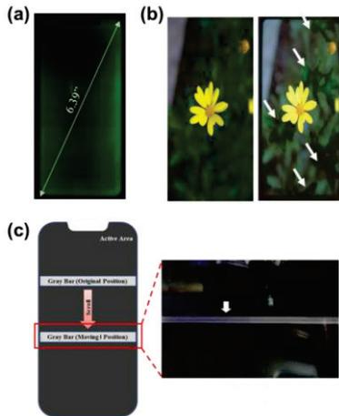
**Fig. 1. 3 types of failure phenomenon appeared at the ultra-low luminance: (a) low gray mura: brighter edge area than center, (b) contour image: color crush which looks like contour, and (c) bluish motion blur: gray bar color change during moving [2].**
