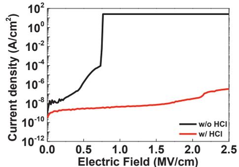
Fig. 2 Leakage current density of Al/HfAlO<sub>x</sub>/p+Si devices without or with HCl
