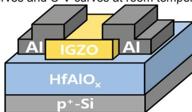
Fig. 1 Schematic of the a-IGZO TFTs using the HfAlO<sub>x</sub> as gate insulator
