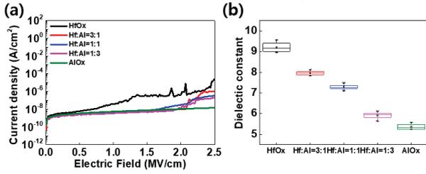
**Fig. 4 (a) Current density and (b) dielectric constant of Al/HfAlO<sub>x</sub>/p+Si devices with different HfAlO<sub>x</sub> film with HCl**
