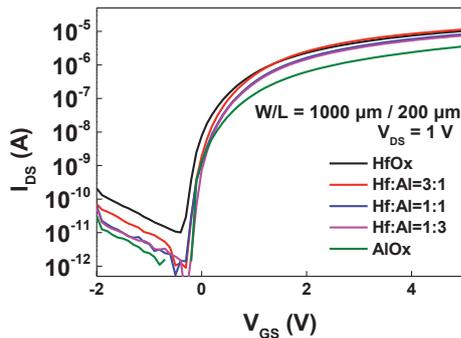
**Fig. 6 Transfer characteristics of a-IGZO TFT with different HfAlO<sub>x</sub> films**
