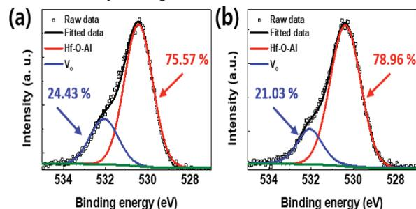
Fig. 3 XPS spectra for O1s core levels from HfAlO<sub>x</sub> films (a) without HCl and (b) with HCl
