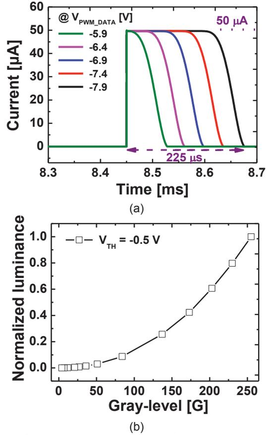
Fig. 3 Simulated (a) current waveforms by varying  $V_{PWM\_DATA}$  (-5.9 V, -6.4 V, -6.9 V, -7.4 V, -7.9 V). (b) normalized luminance of gray-level using 2.2 gamma correction.
