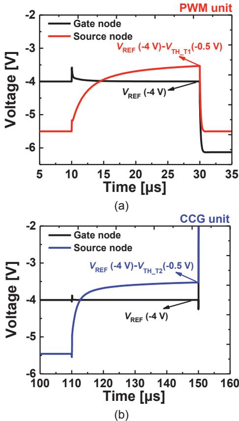
Fig. 2 Simulated voltage waveforms:  $V_{TH}$  compensation in (a) PWM and (b) CCG units.
