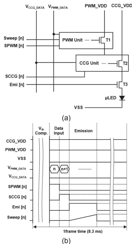
Fig. 1 Proposed pixel circuit (a) schematic and (b) timing diagram
