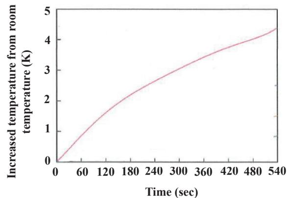
Fig. 4 Temporal change in temperature of the LiNbO<sub>3</sub> crystal during pulse UV laser irradiation.
