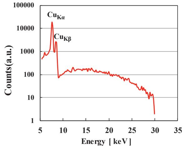
Fig. 2 X-ray spectrum generated by using a Cu target and a LiNbO<sub>3</sub> crystal excited by a pulse UV laser.
