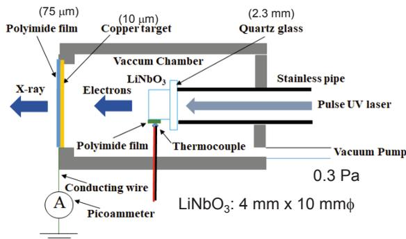
Fig. 1 Experimental setup of the X-ray source
