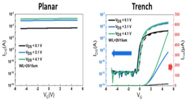
**Fig. 2 Transfer curves of Al-ITZO TFT in typical planar structure and with trench after post annealing @ 230°C**
