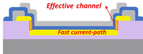
**Fig. 7 Origin of high current in trench TFT**
