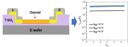
**Fig. 5 I-V Characteristics of channel depending on the  $V_{DS}$**
