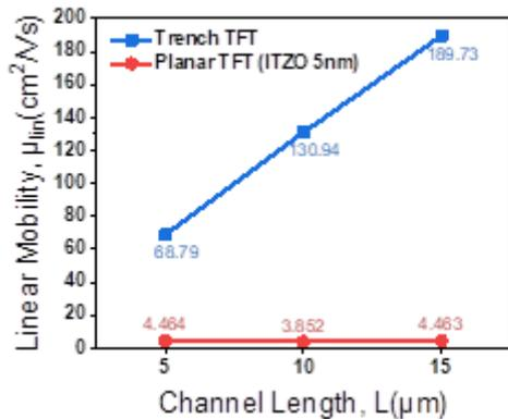
**Fig. 4 Channel length dependence of each TFT**
