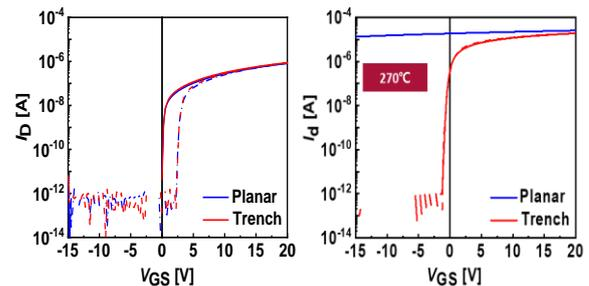
**Fig. 10 Transfer curves of planar and trench TFT fabricated on the same substrate**
