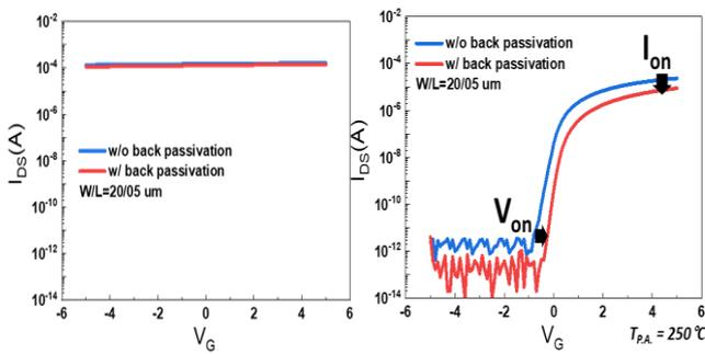
**Fig.7 Effect of back passivation in planar and trench TFTs**
