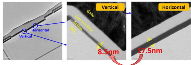
**Fig. 6 TEM image of each part of trench TFT**
