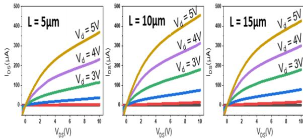
**Fig. 3 Output curves of Al-ITZO TFT with trench depending on the channel length after post annealing @ 230°C**
