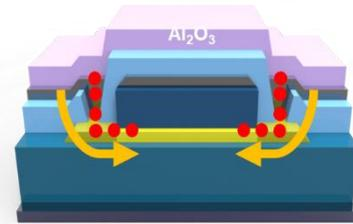
**Fig. 9 Introduction of shallow donor into the channel to induce channel shortening in oxide TFT**
