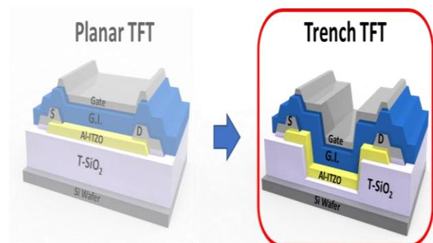
Fig. 1 Schematic diagram of Al-ITZO TFT in typical TGTC planar structure and with trench
