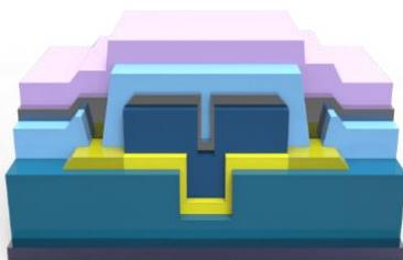
**Fig. 8 Schematic diagram of Al-ITZO TFT in self-aligned structure with trench<sup>5</sup>**
