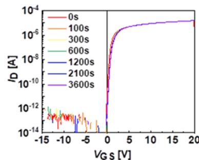
**Fig. 11 PBTS of trench TFT under 1MV/cm at 60 °C**
