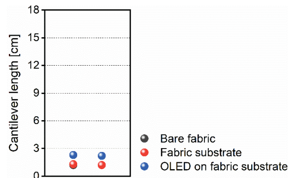
Fig. 4 Cantilever lengths of bare fabric, fabric substrate and the OLED on fabric substrate obtained from the cantilever tests.
