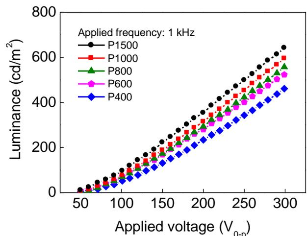
**Fig. 6 L-V characteristics of powder EL**
