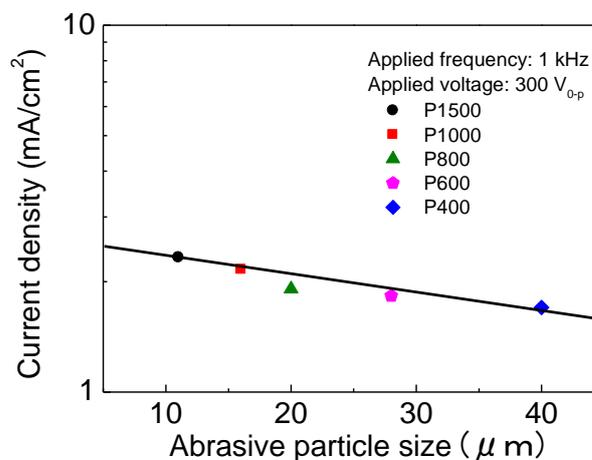
Fig. 4 Current density according to abrasive particle size of substrate
