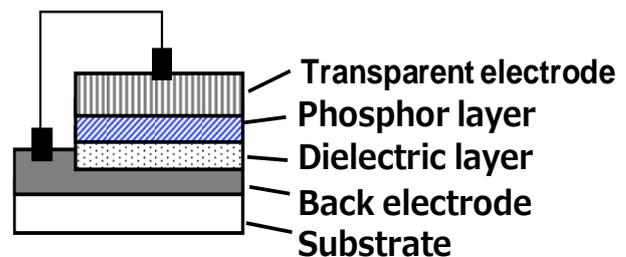
**Fig. 1 Cross-sectional view of the top-emission type powder EL device**
