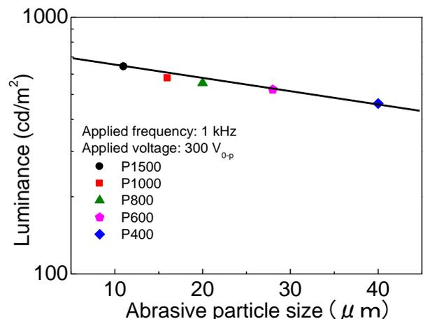
**Fig. 7 Luminance according to the abrasive particle size of the substrates**
