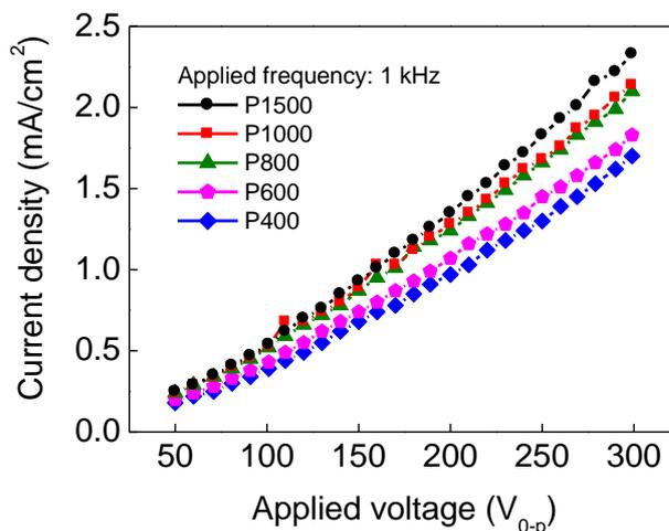
Fig. 3 I-V characteristics of powder EL devices
