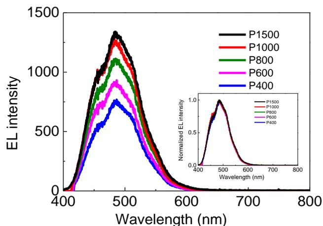
Fig. 2 EL spectra of the devices with different substrates under the application of an AC voltage of 170 V at 1.2 kHz
