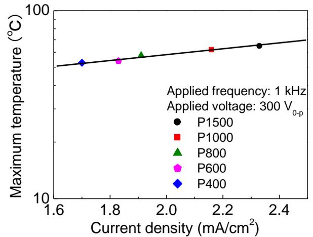
**Fig. 5 Maximum temperature according to the current density of powder EL devices**
