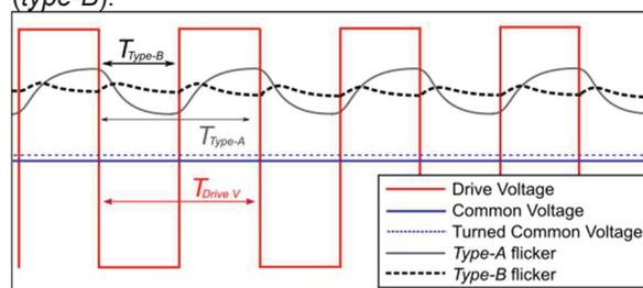
Fig. 1 Drive voltage, common voltage, turned common voltage and flicker types.
