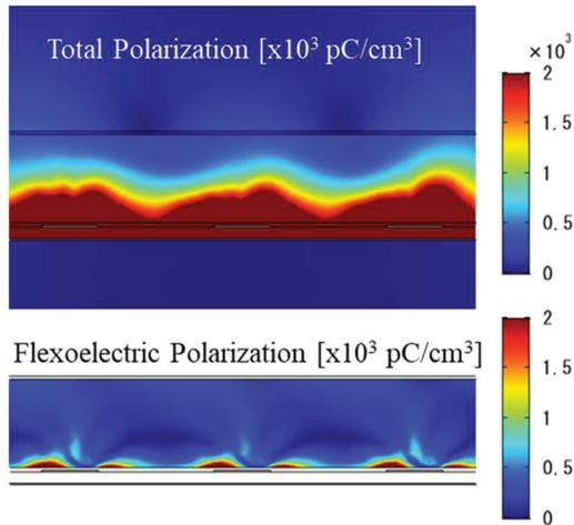
**Fig. 3 Total and flexoelectric polarization densities on TFT drive simulation.**
