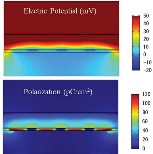
**Fig. 2 Electric potential and polarization density in the FFS-LCD when potential difference between PIX and COM is zero.**
