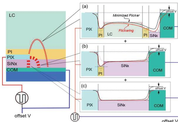
**Fig. 4 Possible electric paths due to the electric properties of FFS-LCD.**
