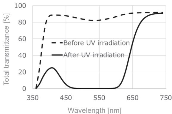
**Fig. 4** Transmission spectrum of photochromic films before and after UV irradiation.
