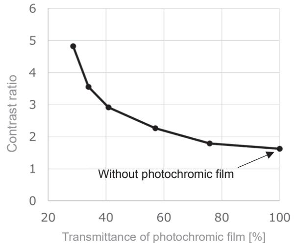
**Fig. 6** Relationship between transmittance of photochromic film and contrast ratio of display photochromic film.
