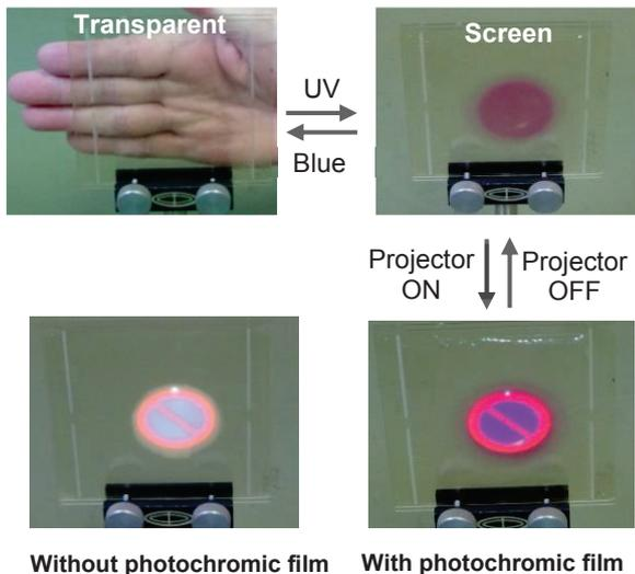
**Fig. 7 Photographs of optically switchable transparent LCD of 10 cm x 10 cm sample.**
