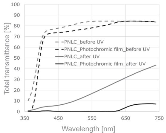
**Fig. 5** Transmission spectra of PNLC and PNLC combined with photochromic film.
