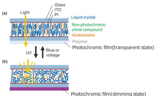
**Fig. 2 Schematic of optically switchable transparent PNLC and photochromic film in (a) transparent state and (b) screen state.**
