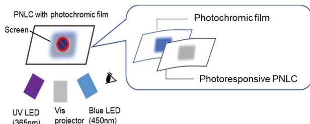
**Fig. 1 System layout of optically switchable transparent LCD combined with photochromic film.**
