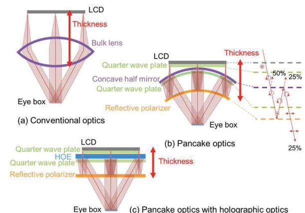
Figure 1. Pancake optics with holographic optics.
