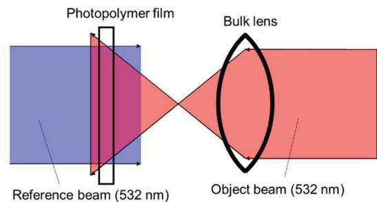
Figure 3. HOE fabrication.
