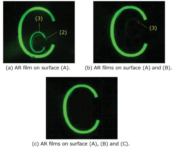
Figure 6. Observed image when AR films were attached.
