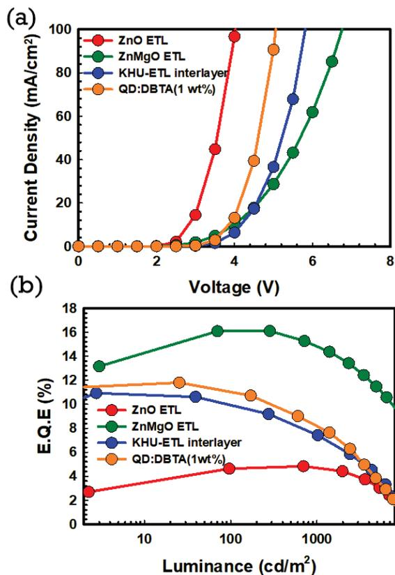
Fig. 2 (a) Current density versus voltage (b) EQE versus luminance characteristics of the fabricated red InP QLEDs devices with ZnO ETL,  $Zn_{0.85}Mg_{0.15}O$  ETL, KHU-ETL interlayer and QD:DBTA(1wt%).
