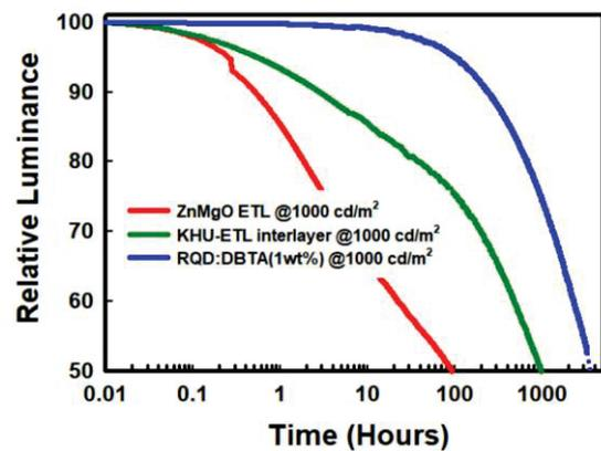
Fig. 3 Operating lifetimes of the fabricated red InP QLED devices with  $Zn_{0.85}Mg_{0.15}O$  ETL, KHU-ETL interlayer and RQD:DBTA(1 wt%).
