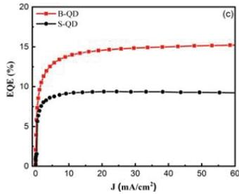
Fig (5) QLED device based on S-QD and B-QD: (a) energy band diagram, (b) J-V-L curves, and (c) EQE-J curves.
