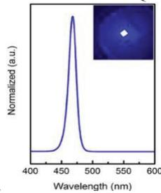
Fig.(8) EL spectrum and image of a QLED device
