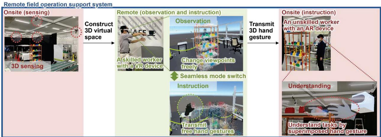
Fig. 1 Remote field operation support system developed in this study.
