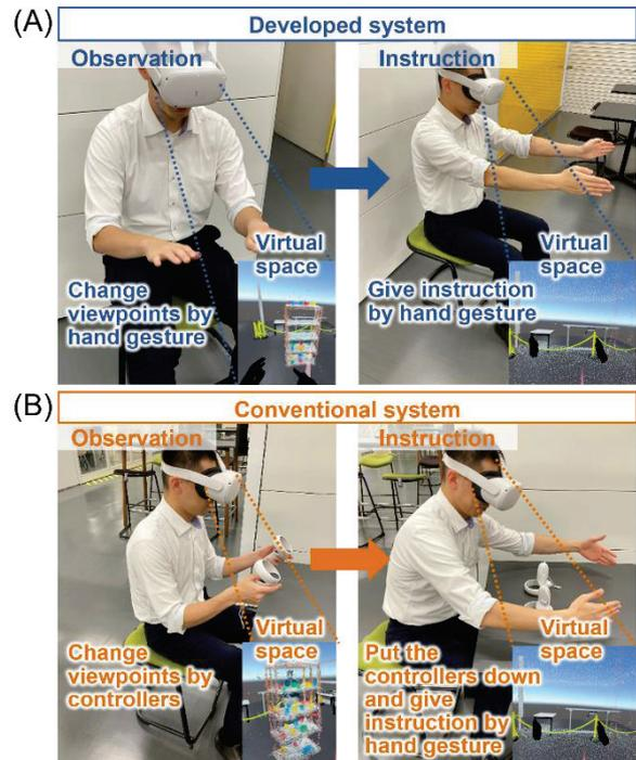
Fig. 4 Experimental conditions. (A) Observation and instruction using the developed system. (B) Observation and instruction using the conventional system.
