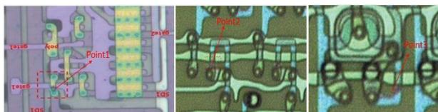
Figure 1. ESD damage location of Poly-Si
