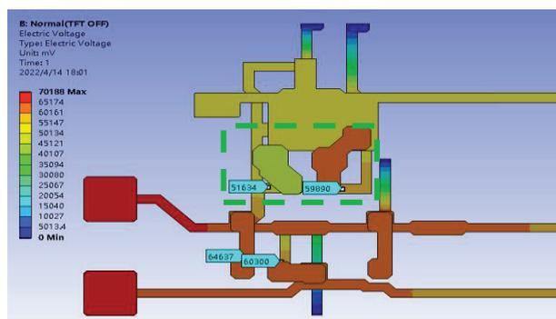
Figure 2. Simulation of electrostatic transmission path
