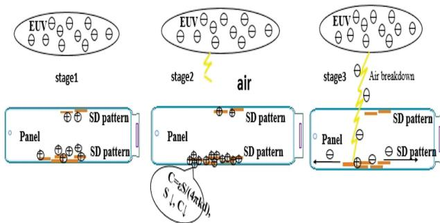
**Figure 3.** Electrostatic mechanism: electrostatic induction, dynamic transmission, electrostatic charge transmission
