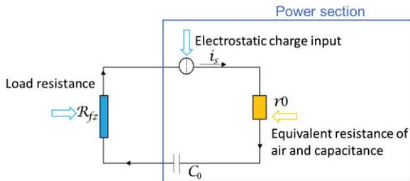
Figure 7. Equivalent electric circuit diagrams
