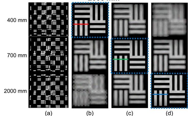
Fig. 7 (a) Generated elemental images by the proposed method and (b)–(d) simulated retinal images focused at 400 mm, 700 mm, and 2000 mm
