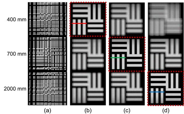
Fig. 6 (a) Generated elemental images by the conventional method and (b)–(d) simulated retinal images focused at 400 mm, 700 mm, and 2000 mm
