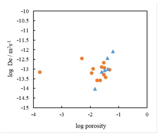
Figure 1 Relationship of logarithmic value of effective diffusion coefficient of uranine versus logarithmic value of the porosity.
