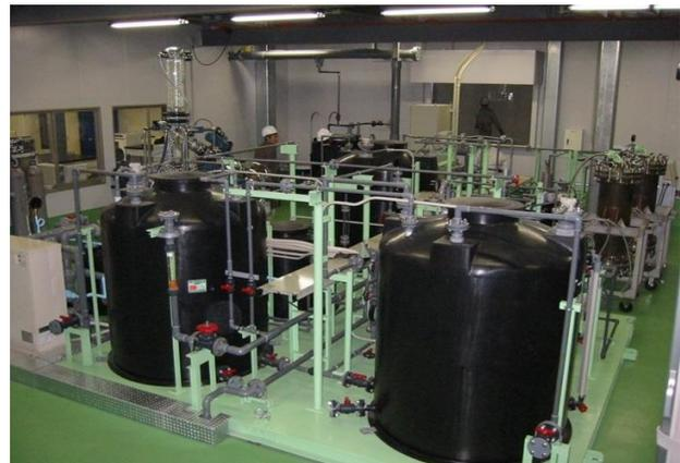
Fig. 7 Pilot plant of lithium recovery from seawater<sup>5-9)</sup>
