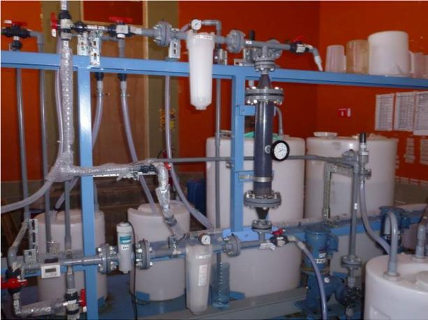
Fig. 11 Benchmark plant of lithium recovery from Salt Lake brine<sup>18,19)</sup>
