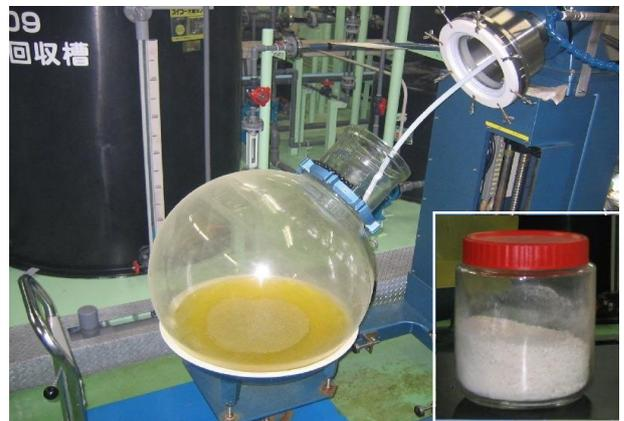
Fig. 8 Concentrated liquid and the dried precipitate obtained by the practical lithium recovery from seawater for 150 days run<sup>5-9)</sup>
