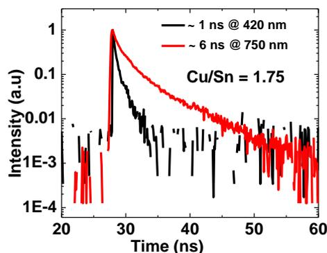
Fig. 2 TR-PL decay curves for bare CZTSSe sample with Cu/Sn ratio of 1.75 at two different excitation wavelength of 420 nm and 750 nm.
