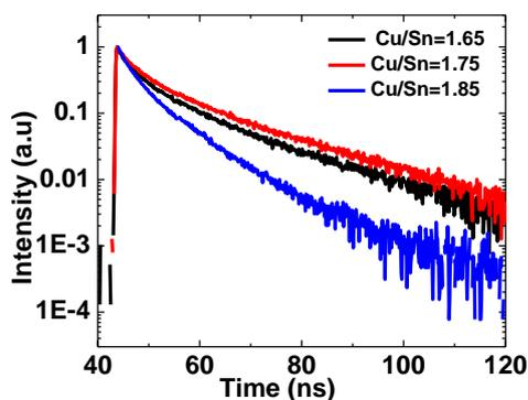
Fig. 1 TR-PL decay curves for CdS covered CZTSSe for three different Cu/Sn ratios under the excitation wavelength of 750 nm.
