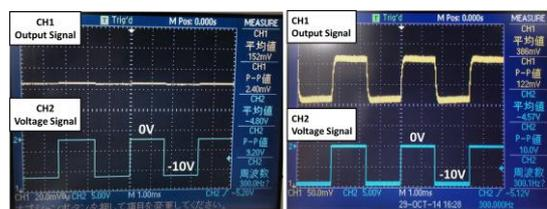
Fig.1 Output signal of the ZnTe bulk device using -10 V pulse function.
