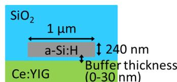
Fig. 1 Cross sectional view of a-Si waveguide on Ce:YIG
