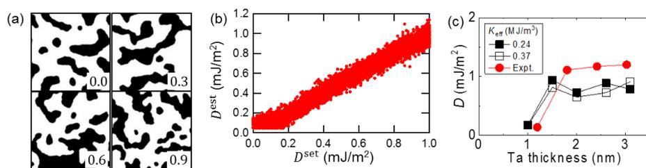
Figure 1 (a) Magnetic domain patterns generated by micromagnetic simulations with each  $D$  value for supervised learning. (b)  $D$  estimated by CNN vs  $D$  set for testing data. (c) Experimental  $D$  values (red circles) and estimated  $D$  values (black and white squares). Data taken from Ref. [1].
