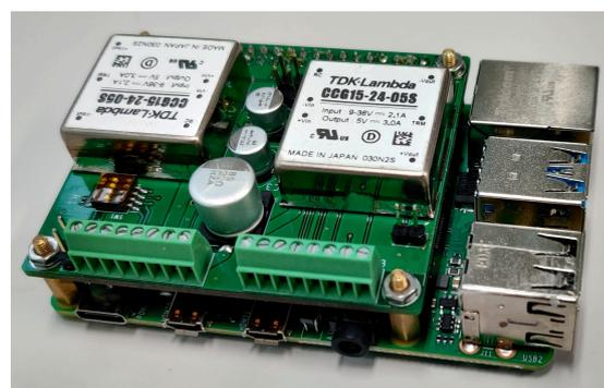
Fig. 2. Manufactured Board with Raspberry pi 4
