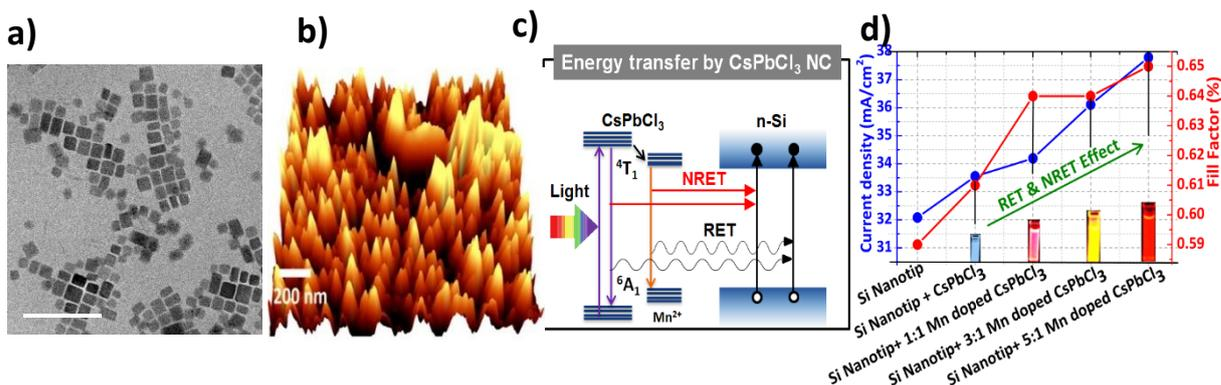
Figure 1 a) TEM image of Mn doped CsPbCl<sub>3</sub> NCs (~100 nm), b) AFM morphology of Si nanotips, c) Schematic band diagram of hybrid organic Si solar cell with Mn-CsPbCl<sub>3</sub> as a downshifting layer and d) the effect of PL spectral tuning and radiative & nonradiative energy transfer of Mn-CsPbCl<sub>3</sub> on the solar cell parameters.
