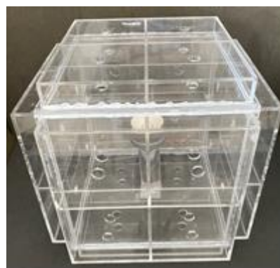
Fig. 2. Photograph of the realized well-ventilated soundproof box.
