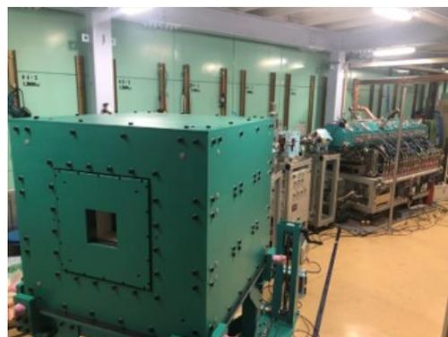
Fig.1 Neutron source RANS-II. In the foreground is the shielding with neutron ejection port. Proton LINAC in the back.
