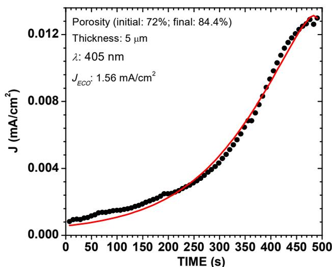
Figure 1: Circles: photocurrent (illumination at 405 nm) during ECO at indicated current density of a PSi layer (initial porosity: 72%; thickness: 5  $\mu\text{m}$ ). Solid line: fit using a model, which will be discussed.
