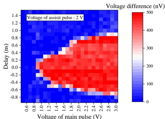
Fig.2. Voltage difference obtained by LFST-FMR as a function of “delay” and voltage level of main pulse.
