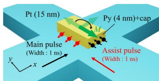
Fig.1. A schematic of device structure for demonstration of SOT magnetization switching.
