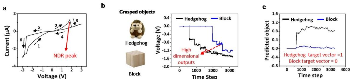
Fig. 1 (a) Non-linear I-V with NDR peak, a redox phenomenon of Por-POM. (b) Right shows the toys grasped by Toyota HSR and left shows the high dimensional spiking time-series outputs generated from hedgehog (black) and block (blue) toys. (c) Test dataset one-hot vector binary classification where the true positive object predicted is a hedgehog (black) with supervised target vector '1' and true negative predicted block (blue) with value '0'.
