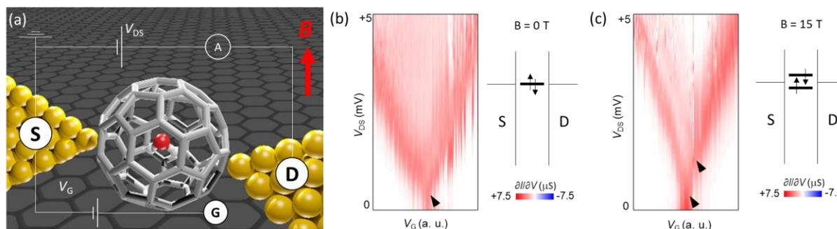
**Figure 1** (a) Schematic of a single molecule transistor (SMT). (b) Coulomb stability diagram of a single-H<sub>2</sub>O@C<sub>60</sub> SMT at  $B = 0$  T. (c) Coulomb stability diagram of a single-H<sub>2</sub>O@C<sub>60</sub> SMT at  $B = 15$  T.
