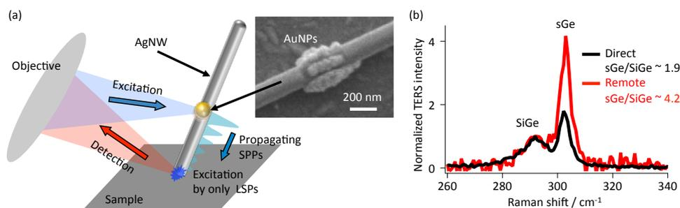
**Figure 1.** A schematic illustration of the remote excitation TERS. Insert is a SEM image of AuNPs on a AgNW fabricated by using the photo-deposition. (b) TERS spectra of SiGe-sGe fin structure normalized at SiGe peak obtained with direct (black line) and remote excitation (red line).
