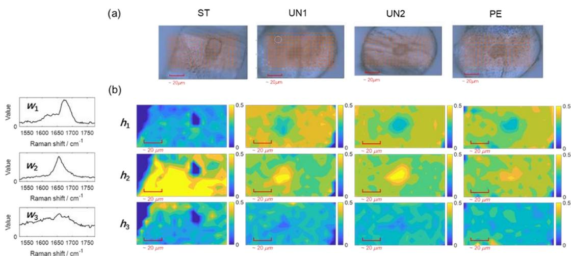
Figure. (a) Visible images of the cross sections of the gray human hair fixed on the quartz substrates. (b) Decomposed spectra  $w_1$ ,  $w_2$ , and  $w_3$  (at the left side) and NMF images of ST, UN1, UN2, and PE constructed by the corresponding scaling factors,  $h_1$ ,  $h_2$ , and  $h_3$  (at the right side).
