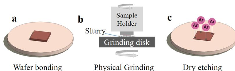
Fig.1. Fabrication process flow. a) Wafer bonding; b) Physical grinding; c) Dry etching
