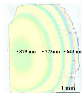
Fig. 2. Completed MOI substrate
