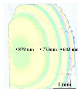
Fig. 2. Completed MOI substrate
